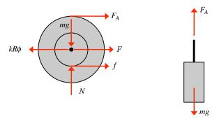
$$\underline{\text{Drum}}: \quad \sum M_C = F(R) + F_A(3R) - kR\phi(R) = I_C\ddot{\phi}$$
