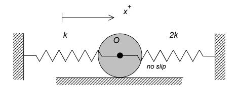
**Given:** A homogeneous disk of mass of m and radius r rolls without slipping on a rough horizontal surface. A spring, having a stiffness of k, is attached between the disk center O and ground, as shown below. A block, also of mass m, is in no-slip contact with the top surface of the disk and with a smooth vertical support at A. A second spring of stiffness k is connected between the block and ground. Let x describe the position of O, where the springs are unstretched when x = 0.
