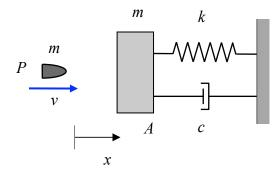
Use the following parameters: v = 10 m/sec, m = 4 kg, k = 3200 N/m and c = 64 kg/sec.
