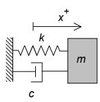
Given: The addition of damping to an undamped system causes the period to increase by 25 percent.
