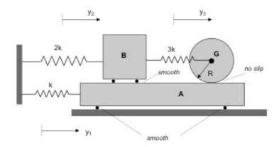
**Given:** The system shown below is released from rest with the initial displacement conditions of  $x_1(0) = x_2(0) = 0$  and  $x_3(0) = A$ .
