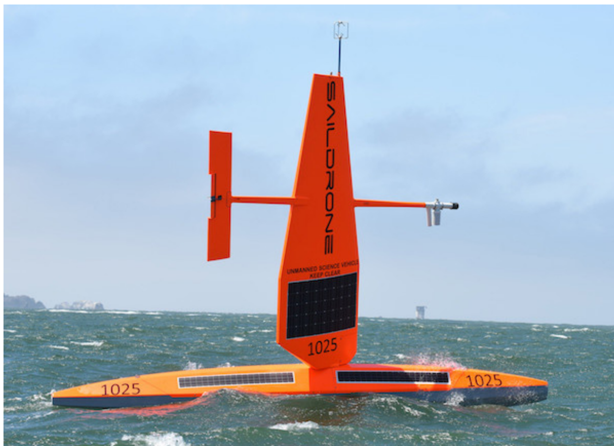
A saildrone maneuvering by wind. Note the solar panels that are used to power the onboard instruments. Photo credit: Saildrone, Inc.
