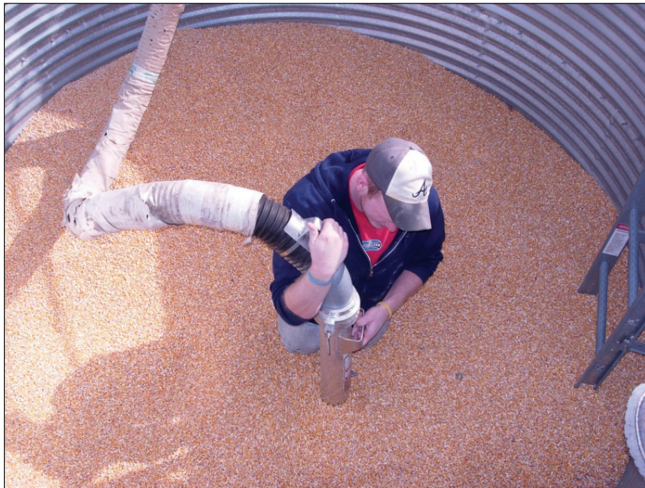
Figure 4. Demonstration of the rate of human entrapment by a grain vacuum system.
