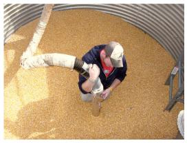
WARNING: Improper use of a grain vacuum machine can result in rapid entrapment.
