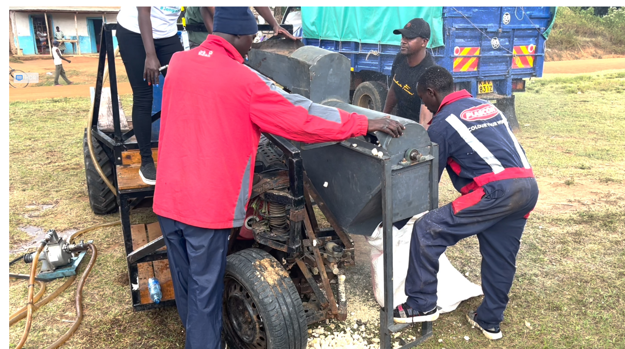
Webuye farmers utilizing the PUP vehicle to help shell corn at a faster rate, May 2023.
