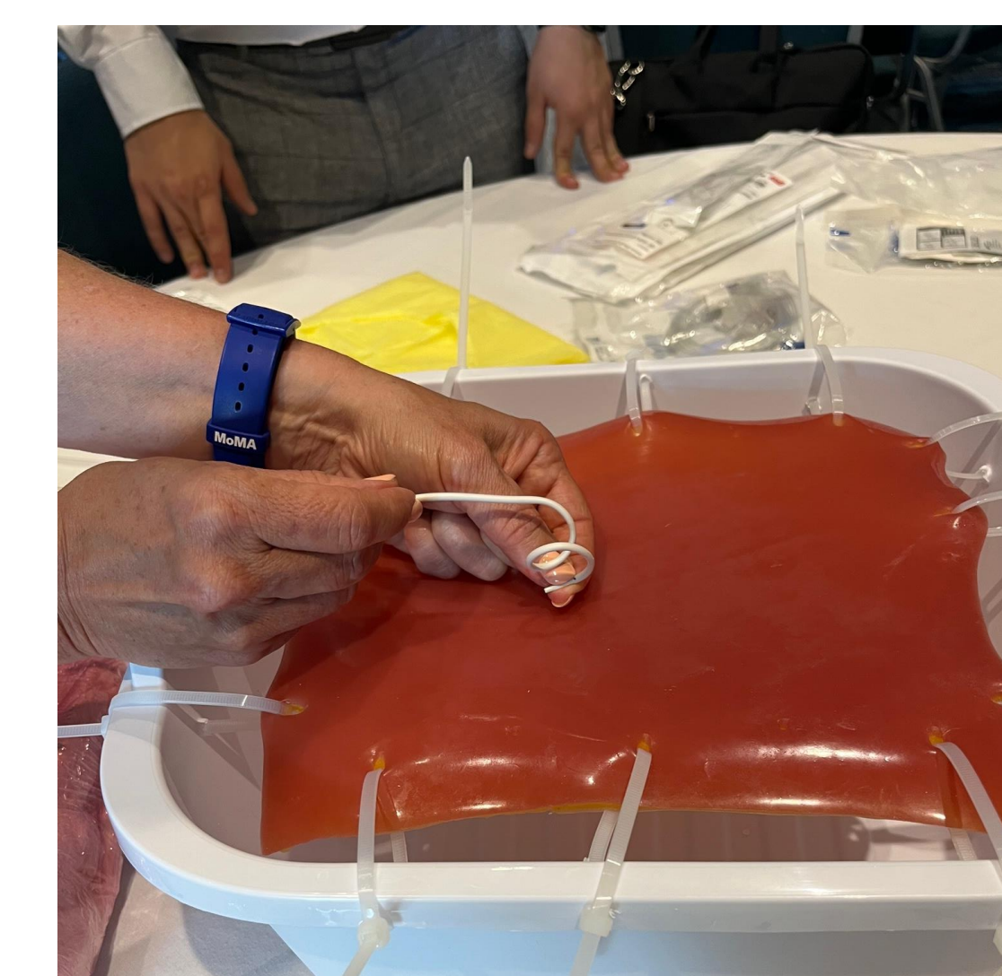
Figure 9. Testing the catheters on a simulated peritoneum similar to those that physicians use in their trainings
