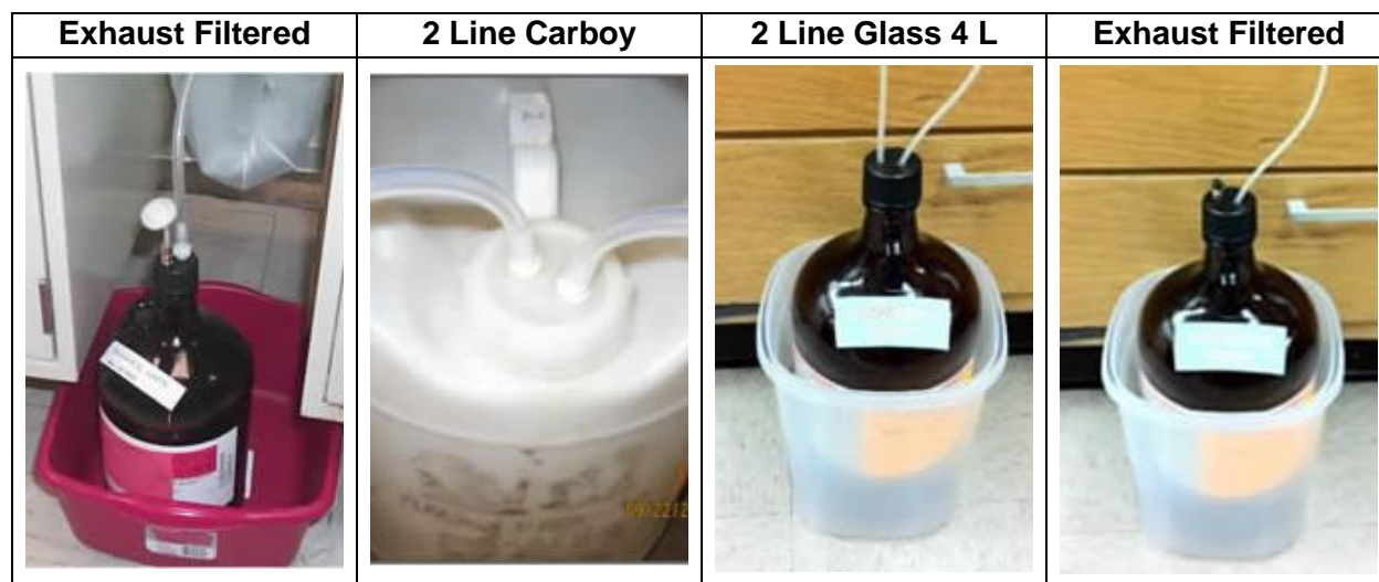
Figure 3.6 – Proper LC Waste Collection with Modified Caps
