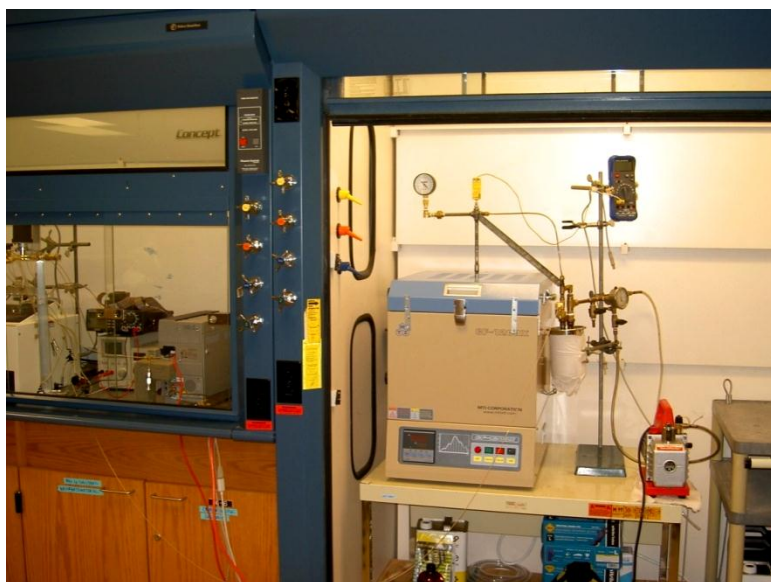
Figure 10: Pyrolysis Test Equipment
