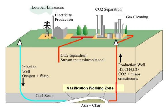
Air is injected into the cavity, water enters from surrounding rock & partial combustion with gasification take place at the coal seam face following ignition. The resulting high pressure syngas stream is returned to the surface, where the gas is separated & contaminants are removed
