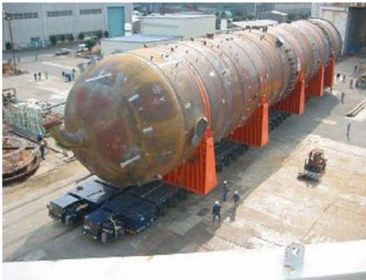
Figure IV.3. Onsite transportation of the Sasol FT Reactor for the Sasol Qatar Oryx GTL Plant (Louw, 2006. The capacity is 34,000 bpd, with 2 FT reactors; each weighs 2100 tons)
