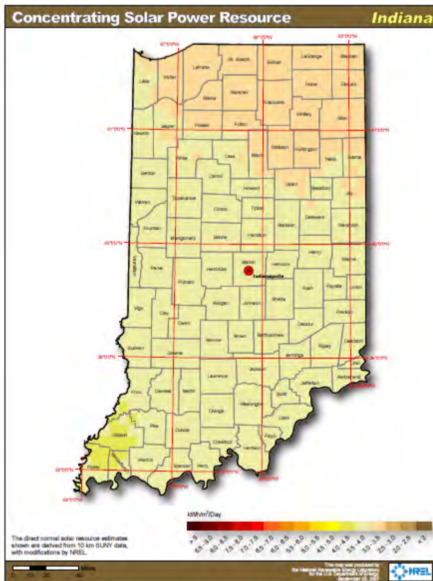
Figure 5-10: Direct normal solar radiation (two-axis solar concentrator) (Source: NREL [15])
