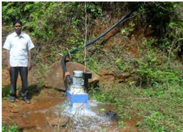
Figure 7-4: Microhydro power facility (Source: Home Power [9])
