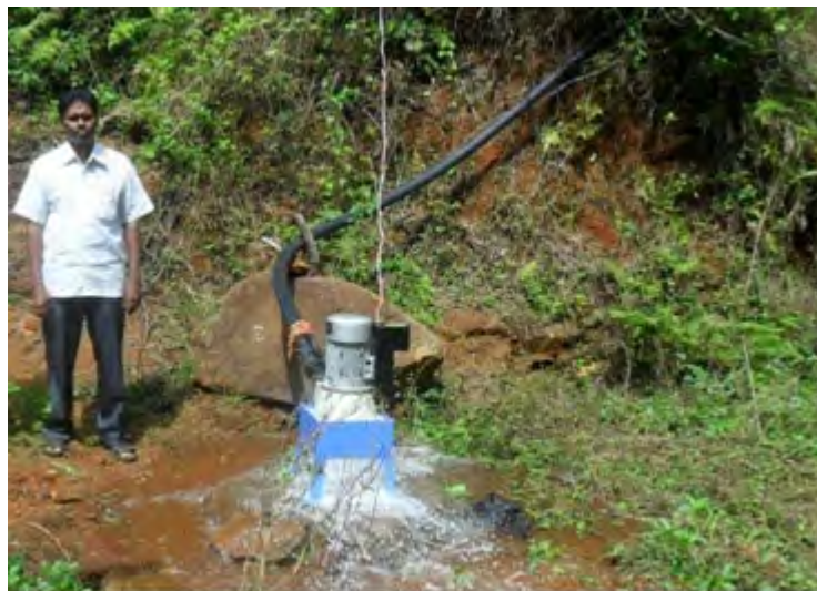
Figure 7-4: Microhydro power facility (Source: Home Power [9])
