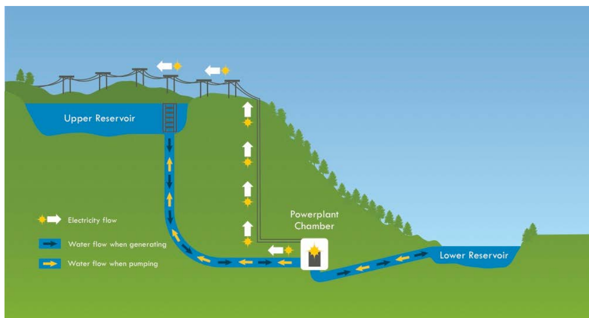
Figure 7-5: Schematic of a pumped hydro facility (Source: DC Thompson and Company [10])
