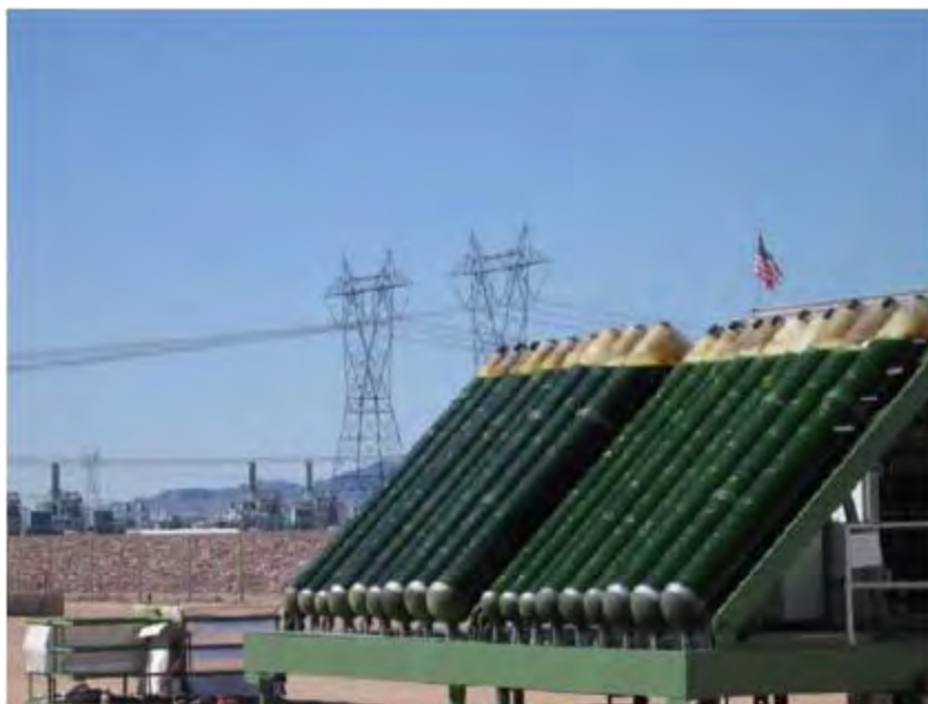
Figure 9-2: Algae bioreactors at an Arizona Public Service power plant (Source: APS: [4])
