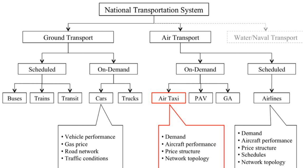
**Figure 1. National Transport System as a system-of-systems**
