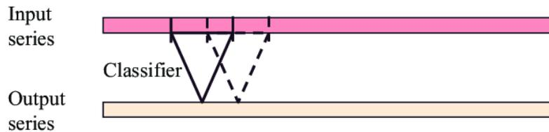
Figure 2: Sliding window scheme for generating a series of predictions.
