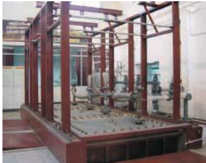
Figure 8. Model rig of UCG at the Chinese University of Mining & Technology (DTI, 2004).
