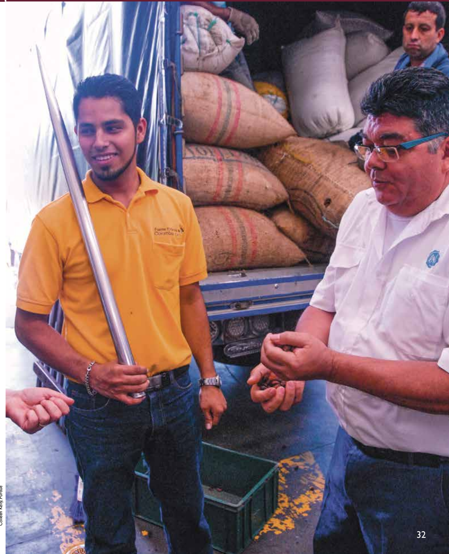
A Nutresa employee perforates sacks of cacao with a hollow metal spike to obtain bean samples in order to perform a quick visual quality check as deliveries arrive.
