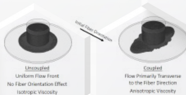
Figure 1: Anisotropic Viscous Flow Compression Molding of a Center Gated Disk
