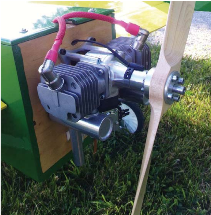
FIGURE 1. 5.5 HORSEPOWER, TWIN CYLINDER OPPOSED, ELECTRONIC IGNITION, TWO STROKE GASOLINE ENGINE
