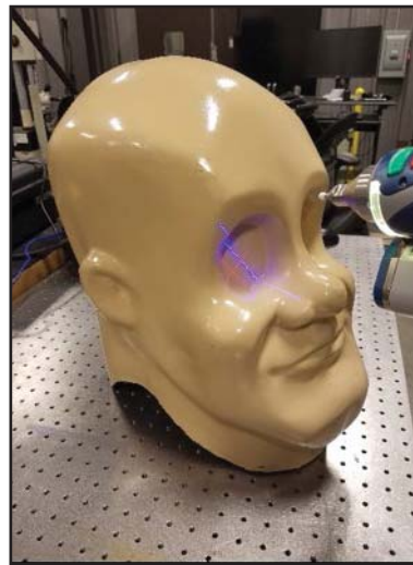
FIGURE 3. PART SCANNING PROCESS.
