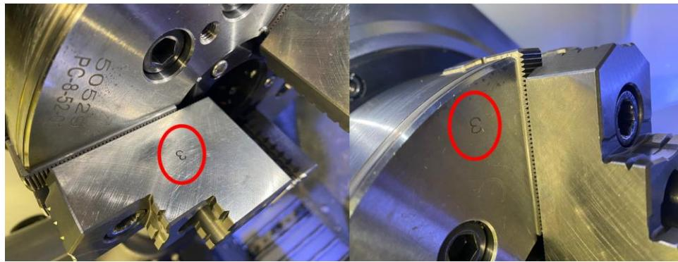
□ Count the number of **TEETH** that are exposed. Use this equation to figure out how many **TEETH** need to be exposed. Negative values are shown in the image below. Ensure all **JAWS** have the exact same **TEETH** count exposed, if not resecure them to match.
