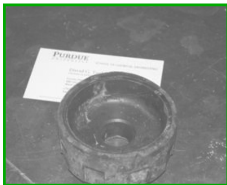
Pictured is the composite top of the autoclave that was sheered off at the threads.
