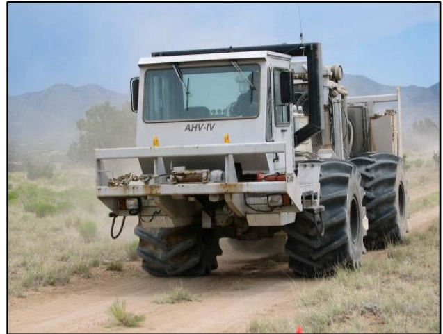
Vibroseis truck provided by ION Geophysical for seismic reflection and refraction data collection at SAGE.
