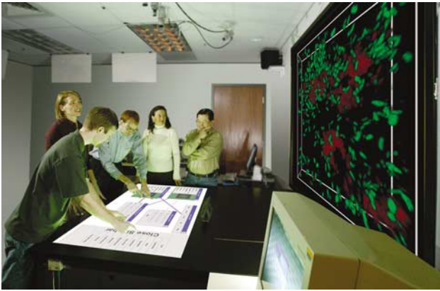
Figure 10 HI-Space users interacting with 3D geometry data generated from 48 confocal microscope image slices at 512 \times 512 resolution.
