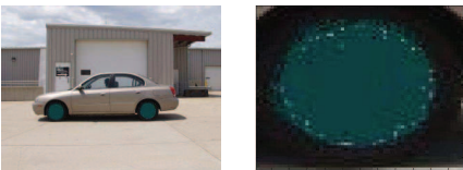
Fig. 16. Result of tire extraction on a vehicle with artificially colored dark tires. The position of the lowermost point of the tire was provided as input.
