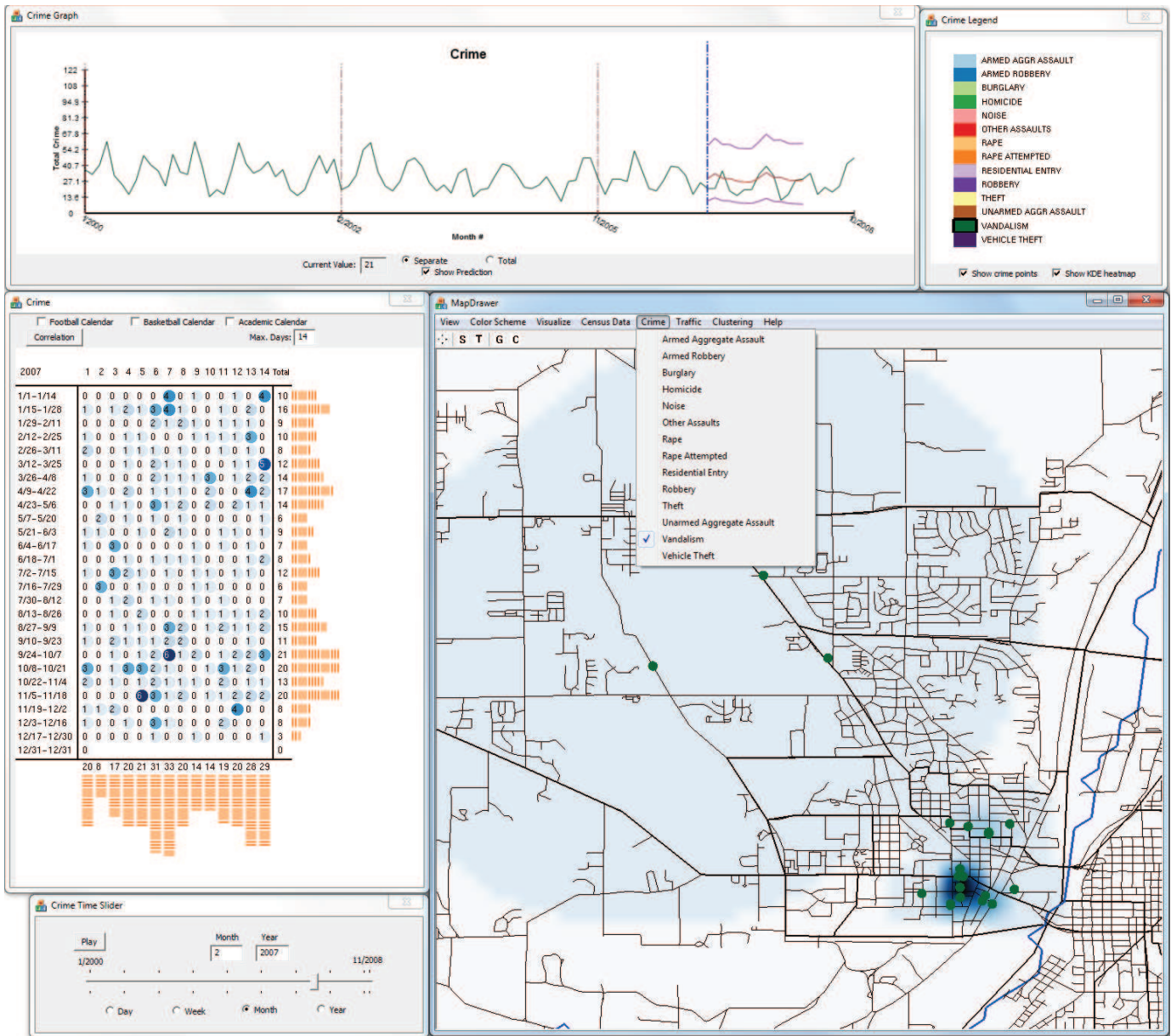
Fig. 1. The Visual Analytics Law Enforcement Toolkit. In this screenshot, the user has adjusted the interactive filter controls (as seen in the map viewing window) to visualize theft. Linked views (above and left) show the line graph and calendar view temporal plots. A legend for the crime incident color mapping is shown in the upper right. The interactive time slider is shown in the lower right. Note the controls for aggregating data by different time scales.
