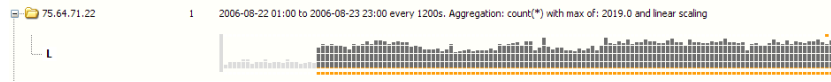
Figure 6. A brushed timeline where the orange highlighting indicates connections to IRC servers on a different port, 6666.
