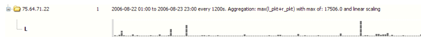
Figure 2. Timeline using an aggregation expression that shows the maximum total packets to and from the local IP that is suspected to be compromised.
