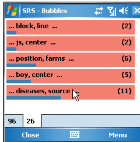
Figure 5. Conversion of cluster visualization as shown in Fig. 4 to a “one-dimensional” view appropriate for a small-screen device.
