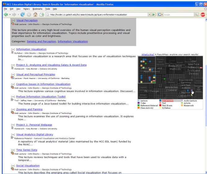
Fig. 4. The effects of brushing a ResultMap node: the corresponding result list item, key entry, and other ResultMap nodes are highlighted. This also shows the result of clicking on a ResultMap node: the corresponding result list entry expands to show additional details and scrolls the viewport to it.
