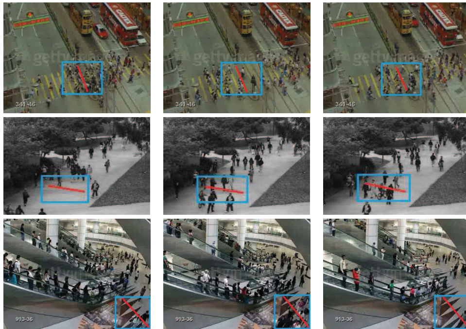
Figure 5. Examples of crowd density estimation on three video sequences. The estimated and true (in parentheses) density levels are (left to right) – Top: 3(3), 1(1), 2(2), Middle: 1(1), 3(3), 4(4), Bottom: 2(2), 3(3), 1(1).
