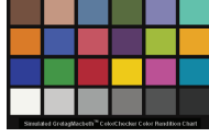
Fig. 3. A printed sheet of colored patches used to construct the camera models.
