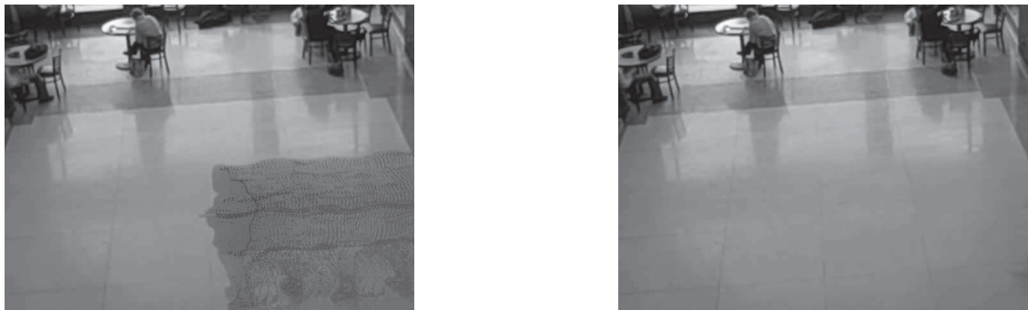
Figure 2. Comparison of the updated background models of frame 138 between a GMM-based method[3] (left) using a constant learning rate and the proposed method (right), the proposed background model reduces the learning rate to zero as the foreground object enters the scene.
