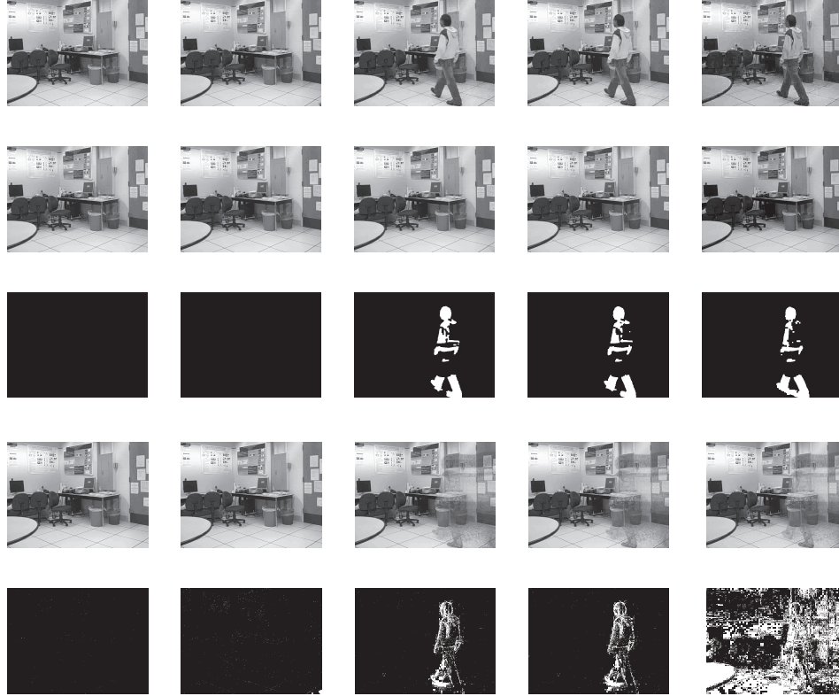
Figure 4. Frame 150, 185, 239, 240, 242 of a sequence with sudden illumination change that occurs between frame 239 and 242, with \Delta I = 22.14 . The GMM method fails when there is a sudden illumination change.
