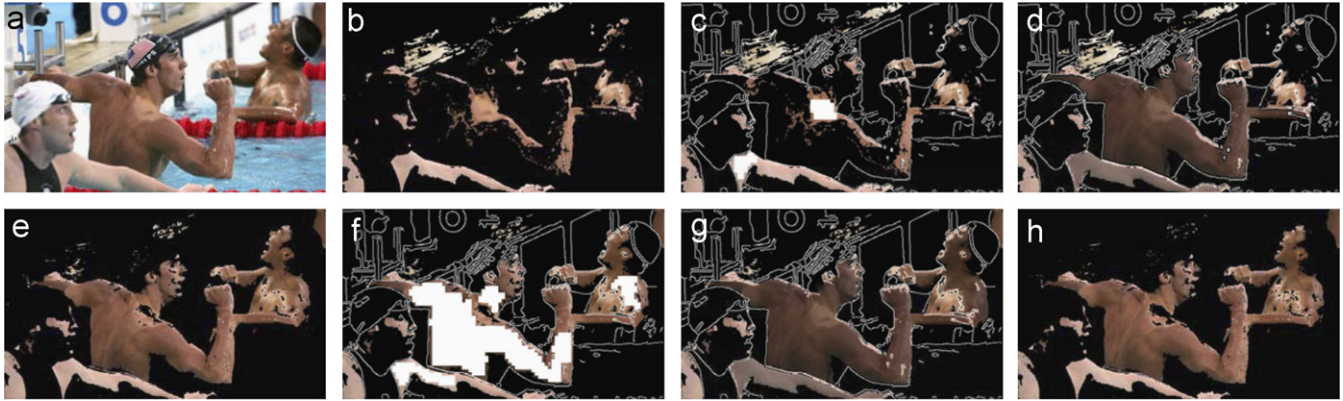
Fig. 4. Incremental learning iterations. Seeded regions are denoted by white patches, and region growing results are denoted by shaded patches. (a) Original image, (b) initial skin map, (c) primary seeded regions, (d) region growing (first iteration), (e) skin map (first iteration), (f) seeded regions (first iteration), (g) region growing (second iteration), and (h) skin map (second iteration).
