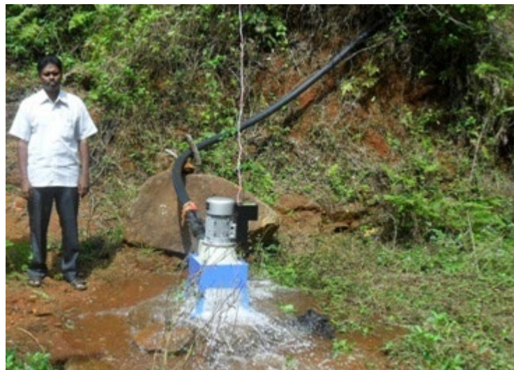
Figure 7-4: Microhydro power facility (Source: Home Power [9])
