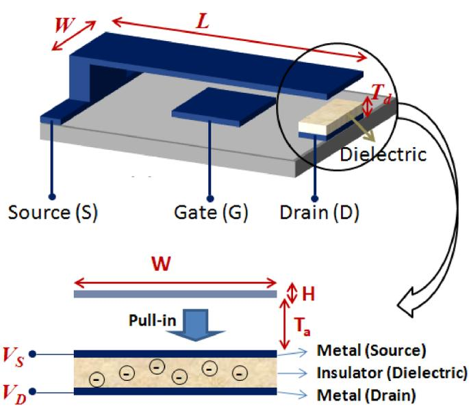
$$\rho WH \frac{\partial^2 w(y,t)}{\partial t^2} + b \frac{\partial w(y,t)}{\partial t} + \frac{EWH^3}{12(1-\nu^2)} \frac{d^4 w(y,t)}{dy^4}$$
