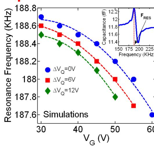
Capacitance of the cantilever RF-MEMS device is measured with varying AC measurement frequency. Resonance frequency ( $F_{RES}$ ) is determined as the frequency of peak in measured capacitance. From simulations,  $F_{RES}$  is found to decrease with increasing  $V_G$  (spring-softening effect) and increasing dielectric charge (increasing  $\Delta V_Q$ ).
