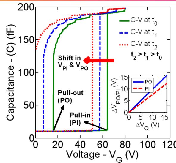
Charge in dielectric is represented by an effective shift in drain voltage -  $\Delta V_Q$ . Presence of non-zero  $\Delta V_Q$  results in actuation voltage shifts of RF-MEMS.
