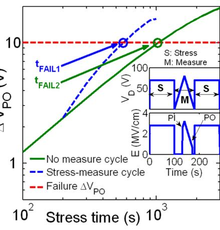
Simulation of a typical characterization procedure for RF-MEMS lifetime using consecutive stress-measure cycles, comparing expected  $\Delta V_{PO}(t)$  with (*Measured*) and without (*Actual*) measure step. The device is said to have failed when  $\Delta V_{PO}$  exceeds a preset value of 10V.
