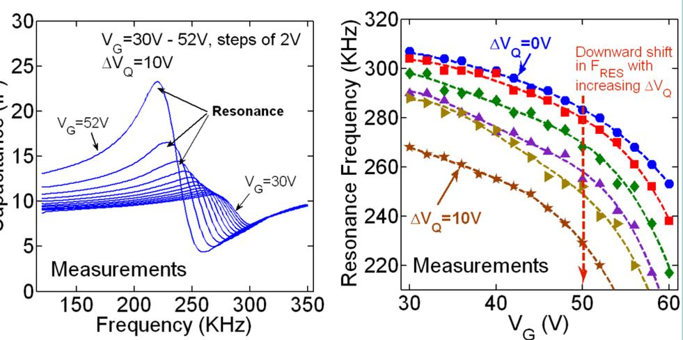
Measurement of capacitance-frequency characteristics of a **packaged** RF-MEMS switch for different gate voltages ( $V_G$ ) and voltage shifts due to dielectric charging ( $\Delta V_Q$ ) were performed to obtain resonance frequencies for each operating conditions. The obtained measurement data is found to have trends similar to those obtained from simulations.
