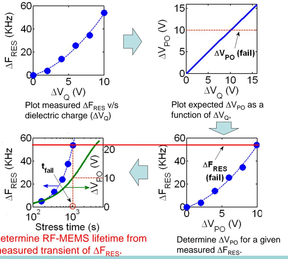
Determine RF-MEMS lifetime from measured transient of  $\Delta F_{RES}$ .
