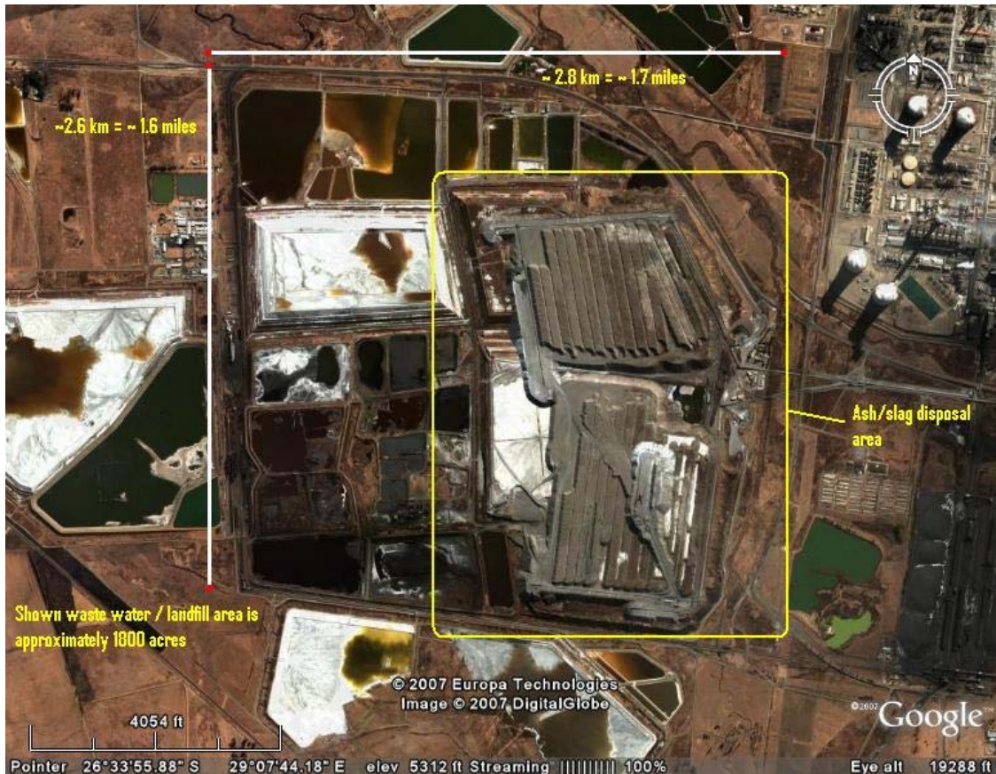
Figure D.12. Ash/slag and waste water disposal areas for the SASOL Plants (Sasol 2 and Sasol 3) in Secunda, South Africa (Source: Google Earth, July 2007)
