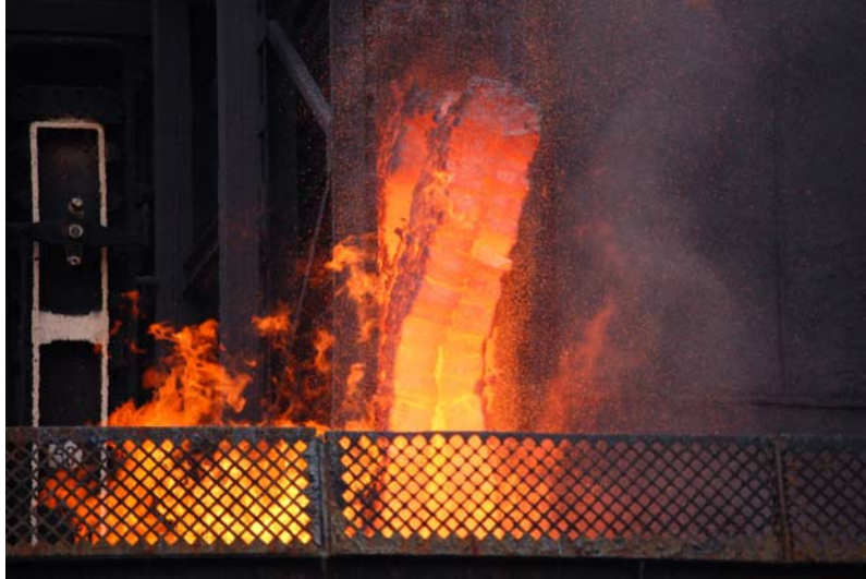
Figure 1: Coke in a Slot Coking Oven
