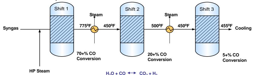
A Water-Gas Shift Reactor converts CO to CO2 with the use of water vapor in the form of high pressure steam. The reaction is exothermic and additional syngas cooling is required
