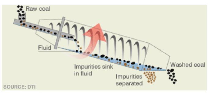
Coal washing involves grinding the coal into smaller pieces & passing it through a process called gravity separation. Technique involves feeding the coal into barrels containing a fluid that has a density which causes the coal to float, while unwanted material sinks & is removed from the fuel mix 10
