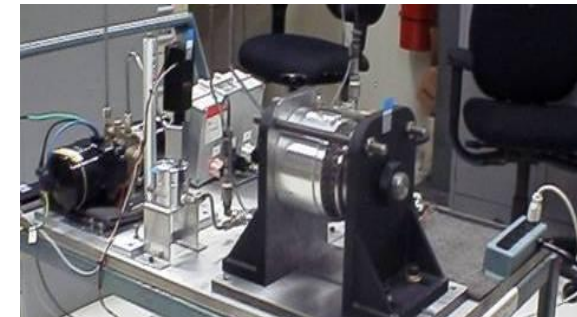
Drive-By-Wire system simulator and On-Demand All-Wheel-Drive system hardware-in-loop bench
