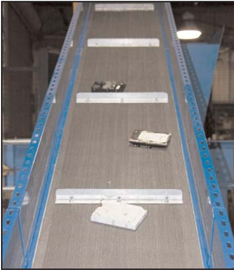
Hard drives are placed on a conveyer belt that will dump them into the shredder.
