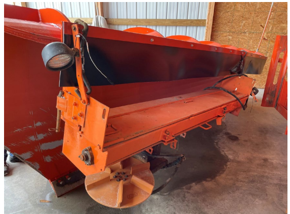
Closeup of Salt Spreader with Chain. Courtesy: White County, IN
