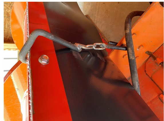
Closeup of Chain that attaches spreader to plow. Courtesy: White County, IN
